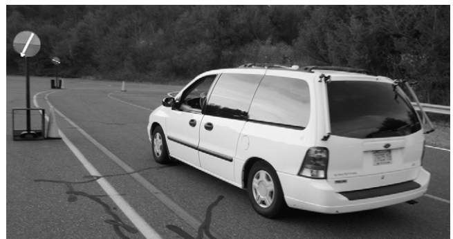
Fig. 1. Pace clocks and instrumented van. Nearest clock currently indicates that driver is permitted to pass.
